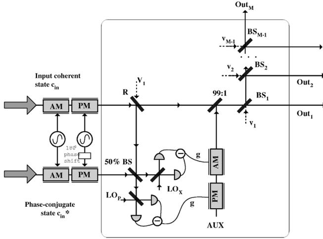
FIG. 1. A schematic diagram of  $1+1 \rightarrow M$  irreversible PCI quantum cloning. BS, beam splitter; LO, local oscillator; AM, amplitude modulator; PM, phase modulator; AUX, auxiliary beam.
