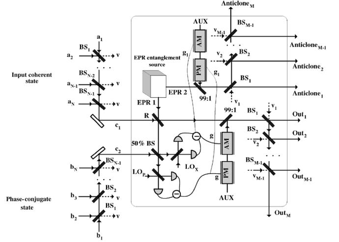
FIG. 3. A schematic diagram of reversible PCI cloning with linear optics and EPR entanglement.
