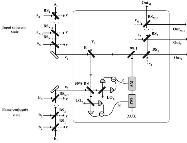
FIG. 2. A schematic diagram of  $N+N \rightarrow M$  irreversible PCI quantum cloning.
